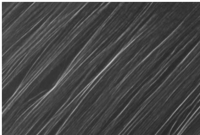
FIGURE 2 Photomicrograph showing optical anisotropy of polymer network in the FLC. The sample was heated to 95°C where the FLC host was in isotropic state. The appearance of the white stripes in the picture results from the light leakage from the polymer stems.
